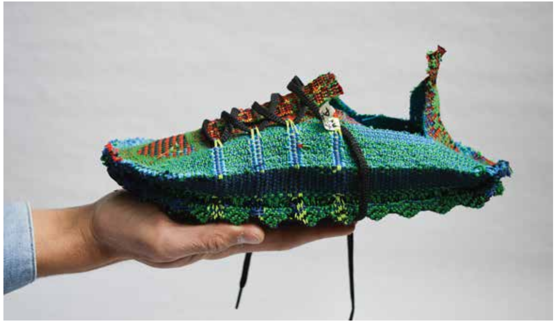
Fig. 1. A 3D-woven shoe: woven in one form on an industrial Jacquard loom. (© VTRG 2019. Photo: Emily Holtzman.)
